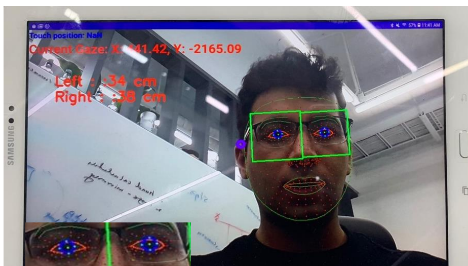
Picture 1: Illustration of accurate iris detection, and distance estimation between a user and a camera. The "Left" and "Right" shows the distance between the user and the device camera in centimeter
