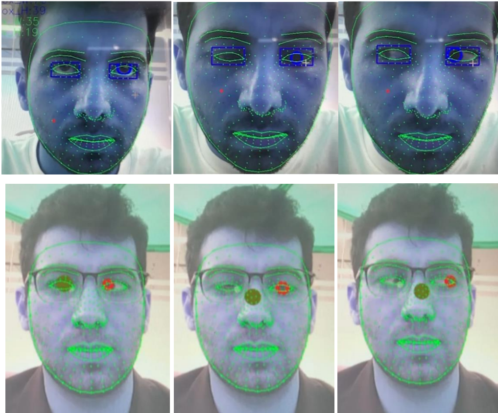
Figure 6: Iris detection using binary thresholding algorithm of OpenCV in combination with mediapipe's facemesh solution.
