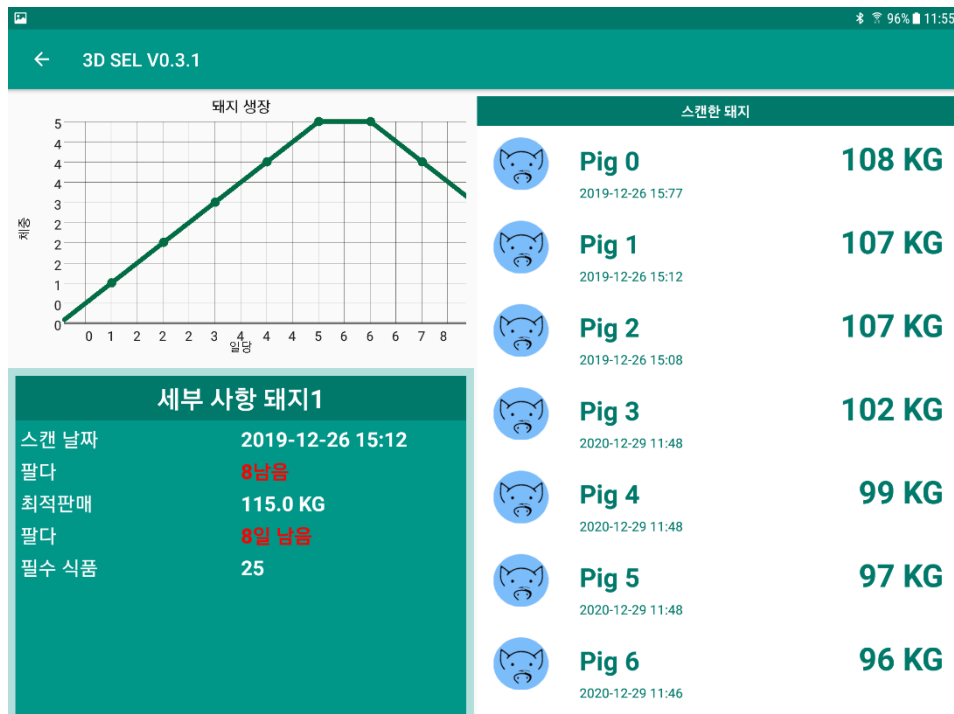
Figure 9: Interactive UI interface: Displays the list of scanned pigs along with its estimated weights (right) and details – date of scan, days left for the optimum sell point, and required food to get to the optimum sell point(left).
